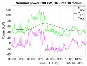
**Figure 1:** ESS mitigating the fluctuating sum power of the PV-wind power system.
