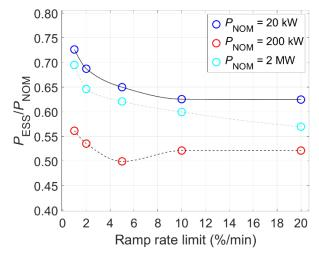
**Figure 3:** Relation between the RR limit and the power requirement of the ESS with different power plant sizes.
