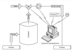
Figure 1. The on-line optical monitoring device.
