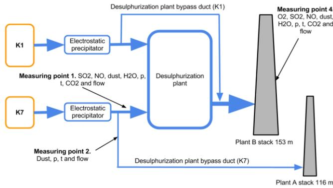
**Figure 2.** Locations of flue gas measurements /7/.
