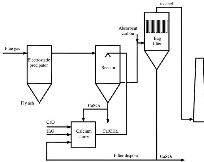
**Figure 1.** Desulphurization process.
