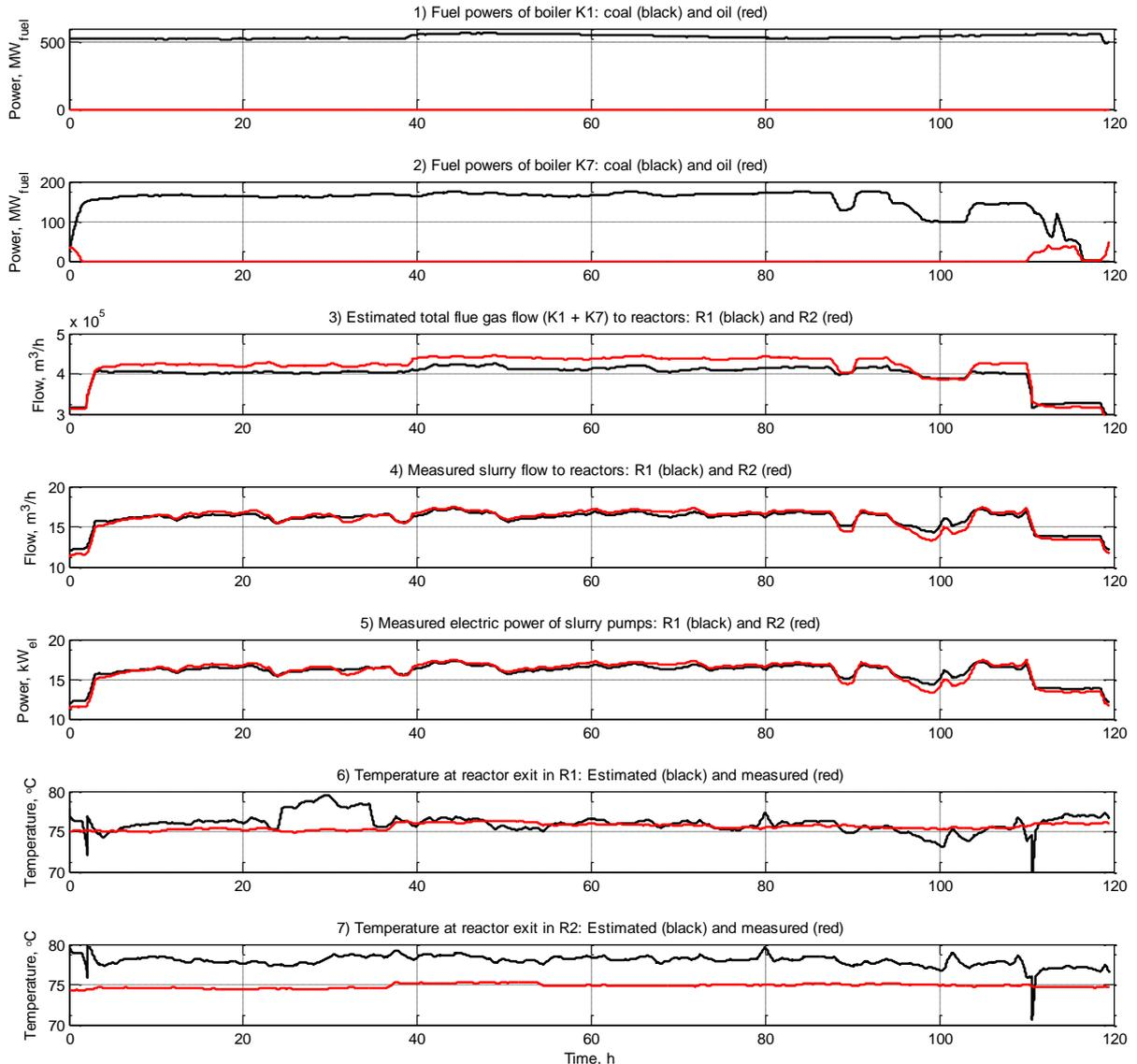
**Figure 3.** Simulation with actual process data. There is a simulated error in Fig. 3.6 at period 25–35 that illustrates situation that 5 % of the liquid in the slurry to R1 do not vaporize.
