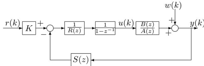
FIGURE 5. Block diagram for the closed-loop system for controlling the process  $B(z)/A(z)$ . The digital controller includes explicit integral action.
