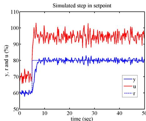
FIGURE 10. Simulated step change in  $r$  for the control systems based on the first model including measurement noise with unit variance. The output  $y$  in blue, actuator signal  $u$  in red and reference signal  $r$  dashed blue.
