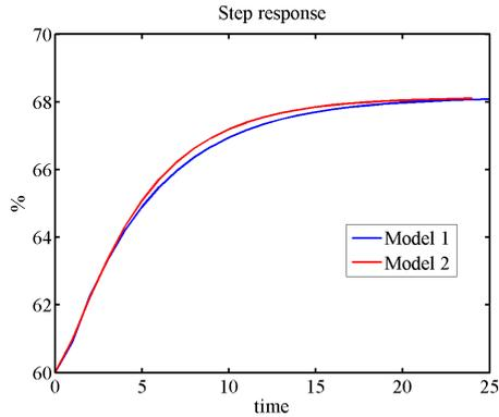
FIGURE 4. Step response for the open loop systems following a change in  $u$  from 70% to 80%. Model 1 in blue and Model 2 in red.
