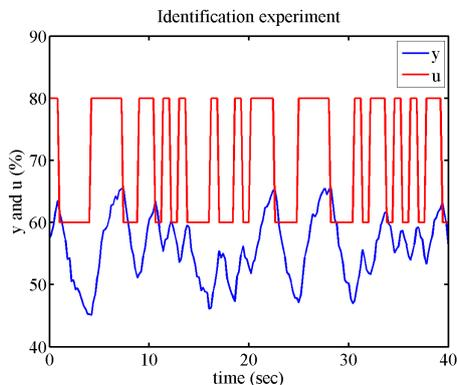
FIGURE 2. Identification experiment, flow,  $y$  in %, in blue, actuator signal,  $u$  in %, in red.
