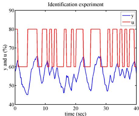
FIGURE 2. Identification experiment, flow,  $y$  in %, in blue, actuator signal,  $u$  in %, in red.
