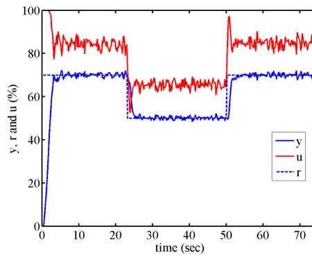
FIGURE 7. Control of the ventilation system for a few step changes using the first controller. The output  $y$  in blue, actuator signal  $u$  in red and reference signal  $r$  dashed blue.
