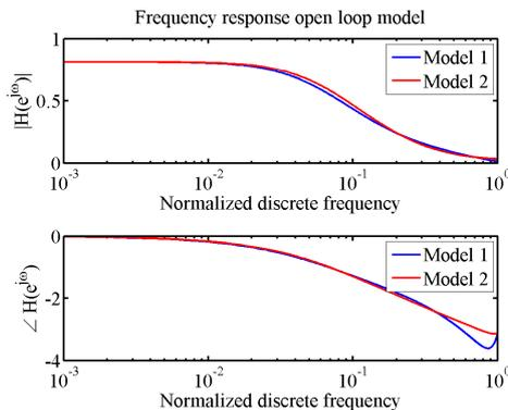
FIGURE 3. Upper panel:  $|H_1(e^{j\omega})|$  in blue and  $|H_2(e^{j\omega})|$  in red. Lower panel:  $\angle H_1(e^{j\omega})$  in blue and  $\angle H_2(e^{j\omega})$  in red
