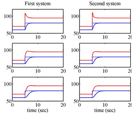
FIGURE 6. Noise-free simulated step changes in  $r$  for the control systems based on the first model (left column) and based on the second model (right column). Upper plots use one pole in 0.7, middle plots have two poles in 0.7 and the lower plots have three poles in 0.7. The output  $y$  in blue, actuator signal  $u$  in red and reference signal  $r$  dashed blue, all in %.
