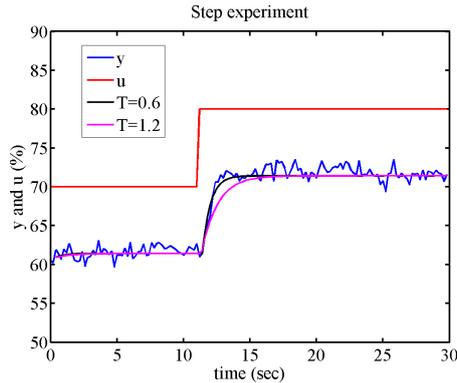
FIGURE 1. Step experiment, flow,  $y$  in blue, actuator signal,  $u$  in red. Simulated step responses using a single time constant,  $T = 0.6$  in black and  $T = 1.2$  in magenta, are included. All signals are provided in %.
