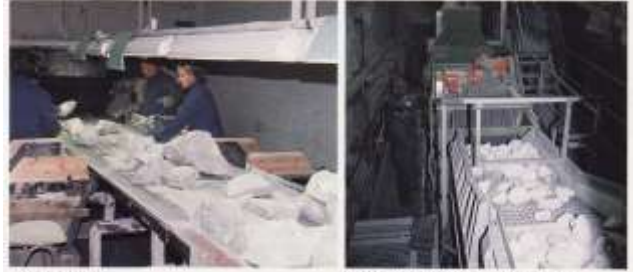
Fig. 2. Manual (left) and automatic (right) sorting of ore.
