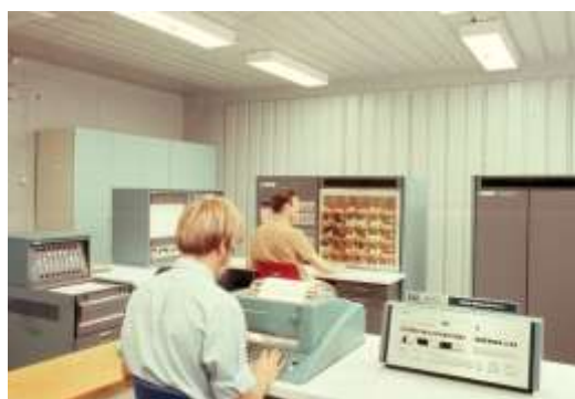
Fig. 1. Hybrid computer used for simulation of the nuclear power plant and the Finnish grid.
