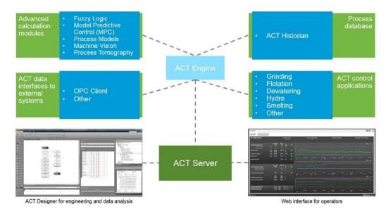
Figure 1. Outotec's Advanced Control Tools platform structure.
