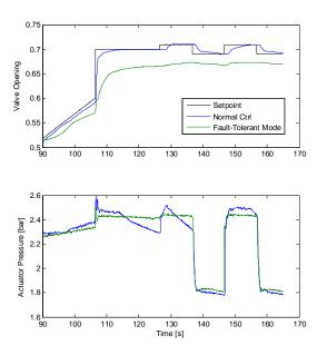
Figure 5. Comparison of control performance with normal control (blue) and with fault-tolerant control (green), which does not utilize position measurement. Above valve opening and setpoint, below actuator pressure.
