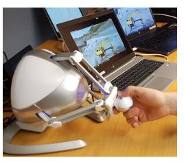
Figure 3. Remote control station with haptic control.
