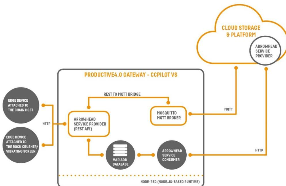
**Figure 1.** Data flow in Productive4.0 use cases and gateway device's software and technology stack.
