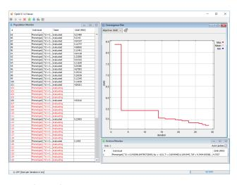
**Figure 2.** The Opt4J graphical user interface. The graph shows the best objective value by each generation.
