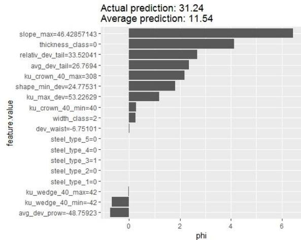
Figure 3. SHAP values for a bad product with a prediction of 31.24, while the average prediction is 11.54 inside the same steel group.
