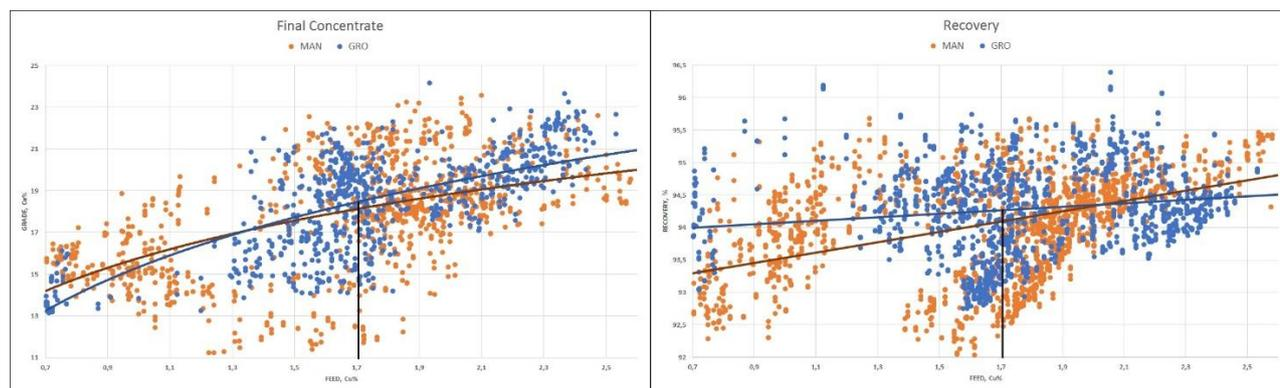
Figure 3. Grade and recovery changes during ON/OFF tests.
