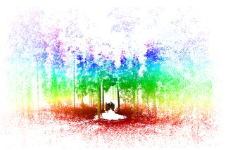
**Figure 3:** A forest machine inside a forest as viewed by the proposed sensor mounted on top of the cabin. The collected point cloud is colorized by the height as hue and point range as value in a hue-saturation-value (HSV) color space.
