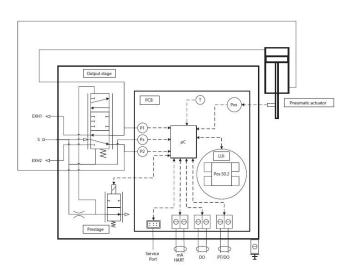
Figure 1. Operating principle of a valve controller.
