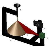
**Figure 1.** Test environment: 1. Video recorder, 2. Laser source, 3. Funnel, 4. Pouring plate, 5. feature marker.
