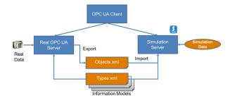
**Figure 3.** Reflection of a Real OPC UA Server with the Simulation Server. OPC UA Clients can connect to either the real or simulation server to get similar data.
