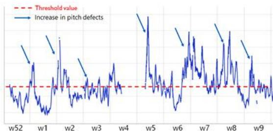
**Figure 4.** Count of colloids versus pitch defects.
