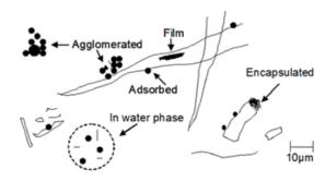
Figure 1. Example of wood pitch in wet end [1].
