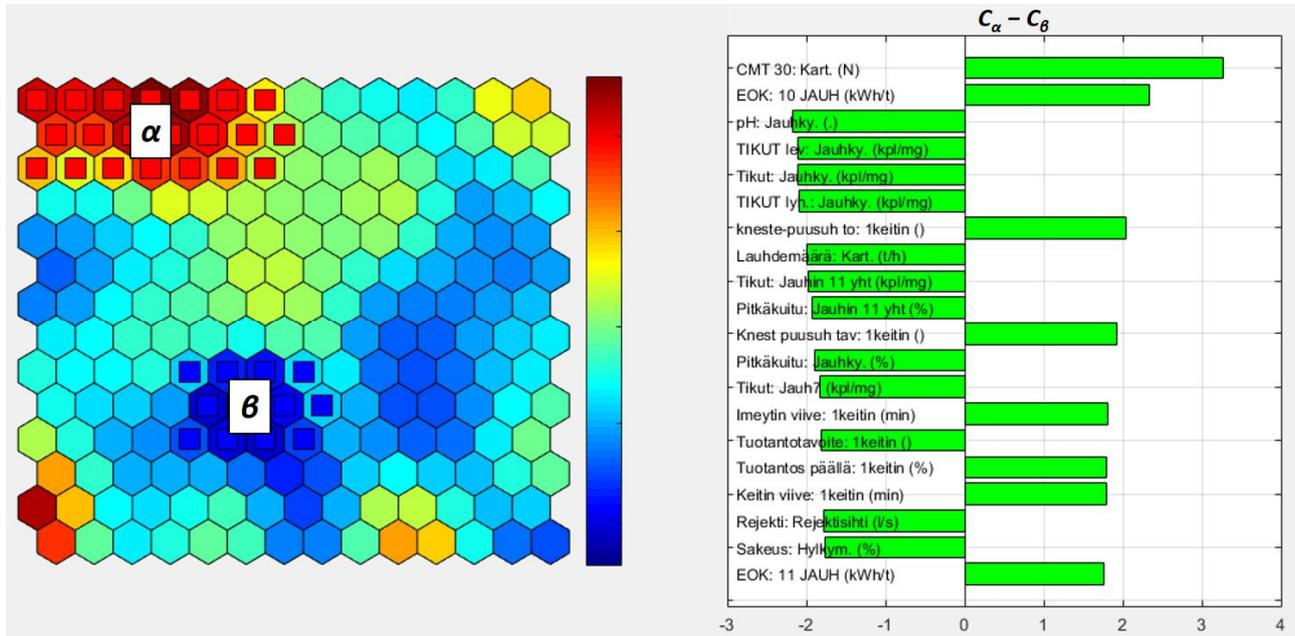
Figure 1. An example of the subtraction analysis in fluting manufacturing. The SOM and the selected areas ( $\alpha$  and  $\beta$ ) on the component plane of fluting quality (CMT) are shown on the left. The color bar indicates the value of CMT on the map (blue = low, red = high). On the right, the result of the subtraction analysis ( $C_{\alpha} - C_{\beta}$ ) is shown.
