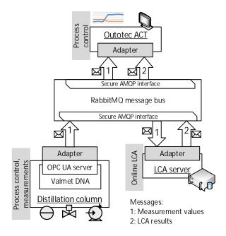
Figure 1. The implementation of the online LCA utilising COCOP communication architecture.
