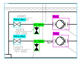
Figure 1. Example of component detection in P&I diagram
