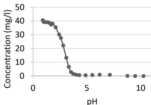
**Figure 1:** Fe<sup>3+</sup> concentration as a function of the pH, calculated by  $R_2$  measurements and the relaxivity presented in Table 1.
