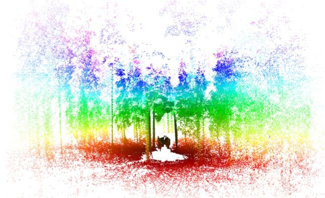
**Figure 3:** A forest machine inside a forest as viewed by the proposed sensor mounted on top of the cabin. The collected point cloud is colored by the height as hue and point range as value in a hue-saturation-value (HSV) color space.
