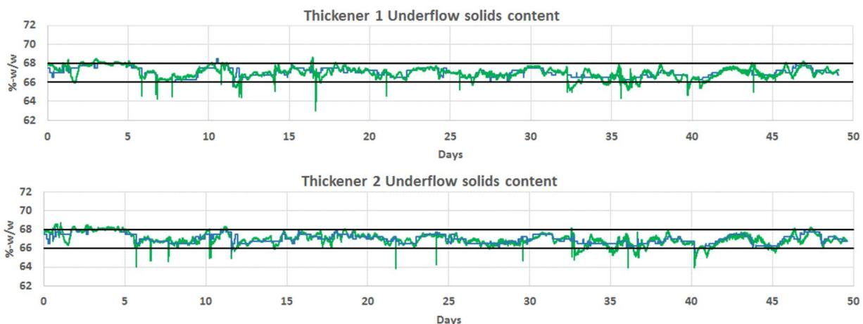
Figure 2. Long-term solids content<sup>3</sup> variability (green: measured value, blue: target value).
