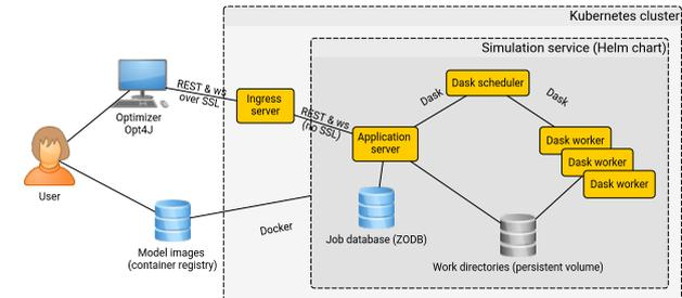
Figure 1. Architecture of the optimization framework.
