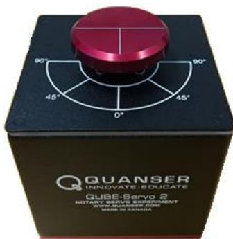
**Figure 1.** Quanser QUBE-Servo 2 unit with disc load.
