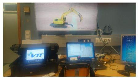
Figure 4. Hardware-in-the-Loop simulator in the remote site.
