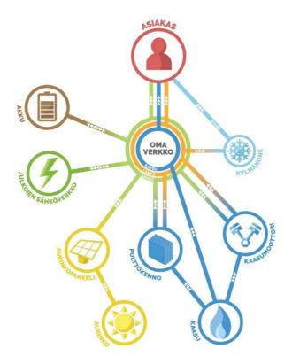
Figure 1. Structure of the Marjamäki microgrid.
