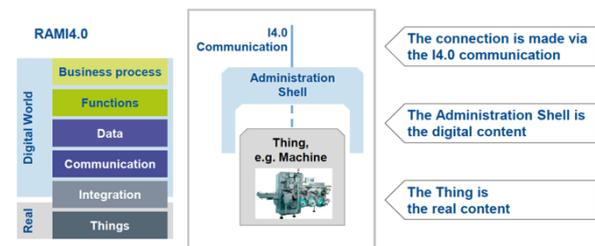
**Figure 1.** Administration Shell is the digital part of an Industrie 4.0 Component.
