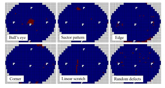
Figue 1: Examples of some typical failure patterns on wafer maps according to literature.
