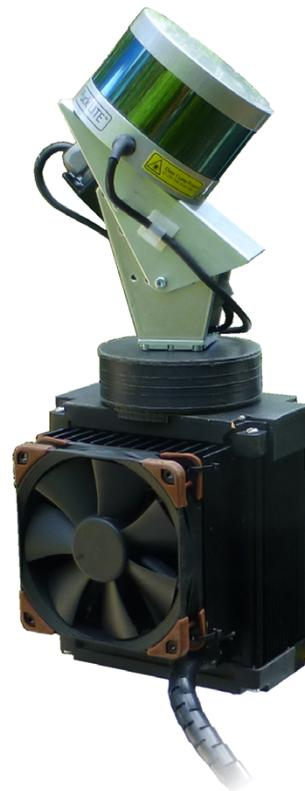
**Figure 1:** A close up of the integrated positioning and mapping sensor
