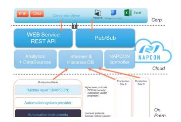
**Figure 1.** Illustrative picture how NAPCON {1] Understand –products can be used for process information collection from various production DCS and IoT sources to cloud corporation analytics utilizing common cloud platforms. All connectivity between sites and NAPCON Cloud is done via OPC UA.
