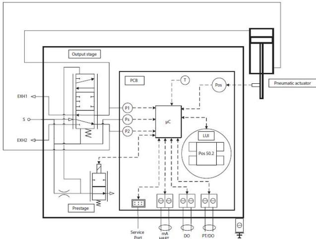
Figure 1. Operating principle of a valve controller.
