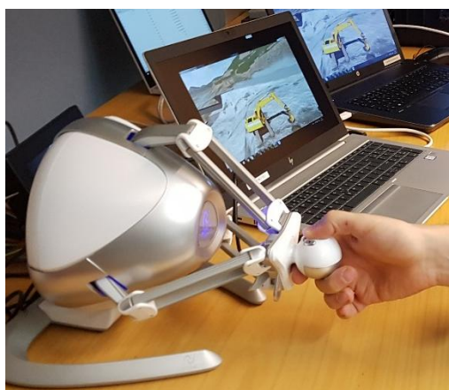
Figure 3. Remote control station with haptic control.
