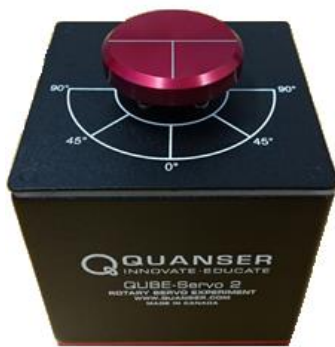
Figure 1. Quanser QUBE-Servo 2 unit with disc load.
