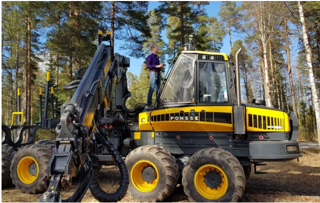
Figure 2: A forest machine and the proposed sensor installed on top of the machine cabin at Evo, Häme Vocational Institute. The corresponding author stands next to the cabin.
