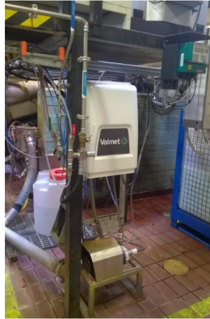
Fig. 5 Valmet LS measures solids in the range of 0 to 5,000 mg/l.
