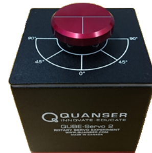
Fig. 2. QUBE-Servo 2 system and a metal disc load.
