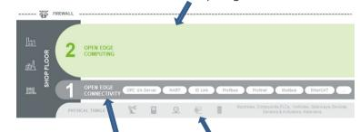
The Connectivity Layer allows connection to non-Ethernet based assets
