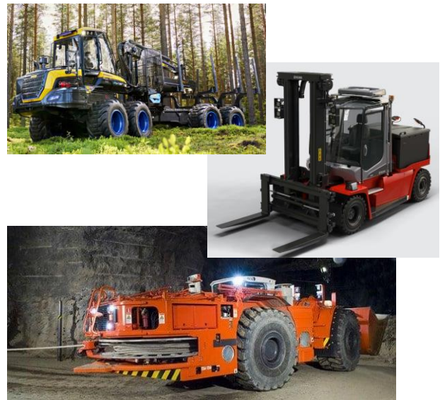
Figure 1. Examples of NRMM electrification: Ponsse hybrid forwarder [3], Kalmar battery-electric forklift truck [4], and Sandvik cable-electric loader [5].
