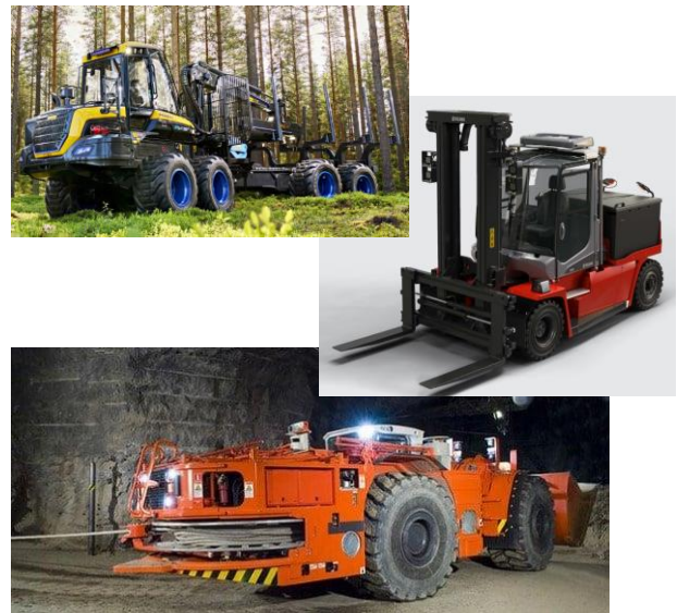
Figure 1. Examples of NRMM electrification: Ponsse hybrid forwader [3], Kalmar battery-electric forklift truck [4], and Sandvik cable-electric loader [5].
