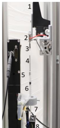
Figure 1: The experimental setup for robotic fiber fabrication. The force sensor is fixed on a frame, and the Dextran dispenser is mounted on a motorized precision stage.
