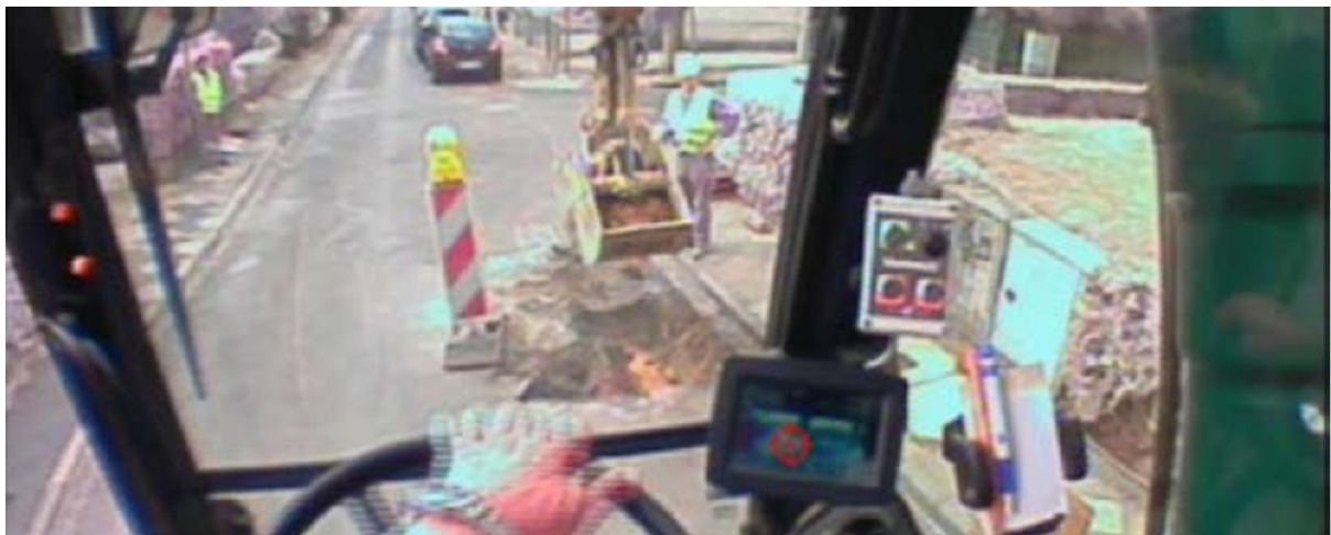
Figure 1. Operators' glance to CMS (fixation identified by eye tracking) during operations with mobile excavator.
