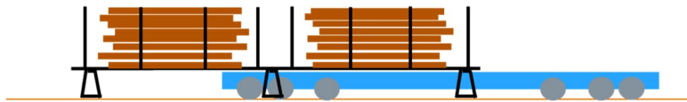
Figure 1 An outline of the situation where the autonomous vehicle drives under the full saw log cage
