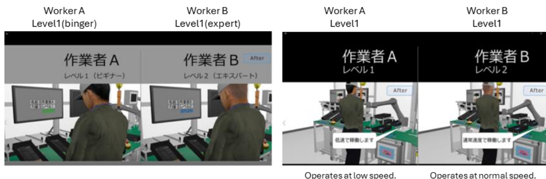
Fig. 6 The robot operates at a set upper operating speed limit (SLS function) according to the operator's competence.
