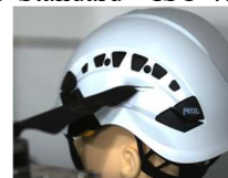
Figure 10 Propeller penetrating the helmet. Standard: EN397, Propeller: 20 in
