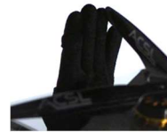
Figure 5 Finger not amputated. Standard: EN388 Level 1, Propeller: 15 in
