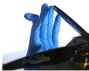
Figure 4 Finger amputated. Glove: N/A, Propeller: 15 in
