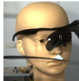
Figure 7 Eyewear dislodged. Standard: ANSI Z87.1+, Propeller: 15 in
