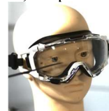
Figure 8 Eyewear not broken. Standard : ISO 4007, Propeller: 20 in
