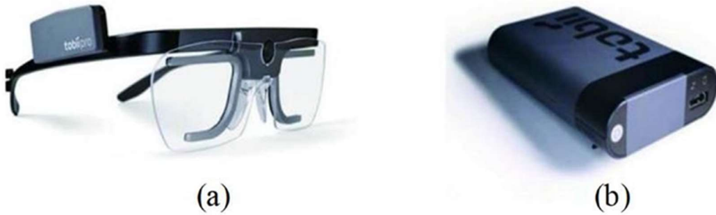
Figure 2. Eye-tracking experimental setup consisting of (a) a data acquisition unit and (b) a data recording unit [5]
